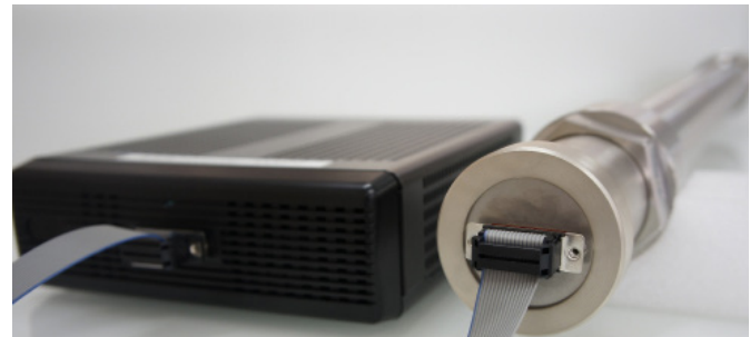
Figure 1: The detector is powered by 12 V through a control unit. TTL output is available as well as ToT histograms and neutron count rates. Multiple detectors can be connected to large arrays.
